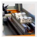
Manual precision holder with variable workpiece holding
