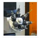
Turret head for 6 WF-35-series tool holders, horizontally mounted, spindle speed 10 000 min<sup>-1</sup>, rotation from tool to tool (60°) with torque servo motor in approx. 1 sec.
