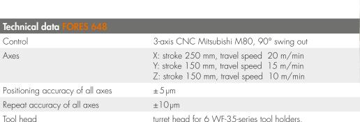
turret head for 6 WF-35-series tool holders, turret rotation by torque servo motor, 60° in ~1 sec., pneumatic stop
